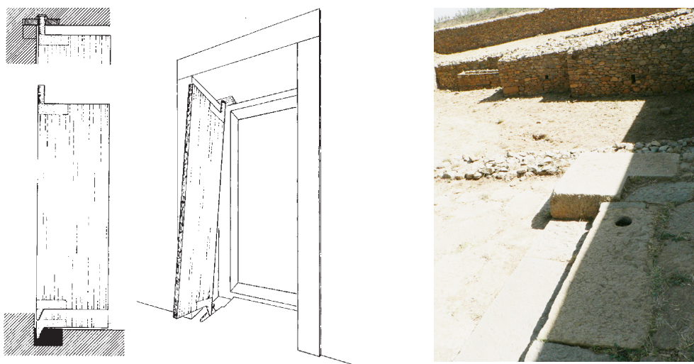
Fig. 2 (Left): Reconstruction of an Aksumite door with the "Türangelstein", the hole serving as a hinge for the door (by the author).
